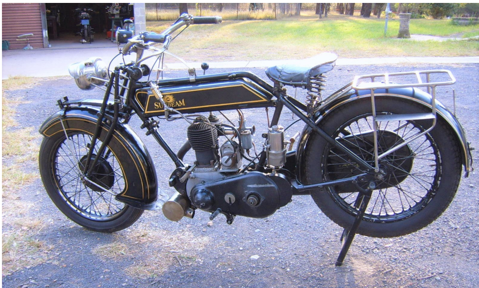
1919 Sunbeam 3 1/2 h.p. described in Rick Nabkey's letter. Front brake is non-standard. Note interesting leaf spring front suspension.
