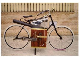
Manuel was kind enough to send over several photos and a description of the bike. Guillermo began with many original 1896 parts, including a Columbia Pope bicycle frame, seat, fork, handlebar and hubs. The team also sourced a period pressure gage, taps, valves, etc. so that the bike seems very authentic. Many parts were blacksmith and locksmith fabricated and also cast via the Galicia foundries.
